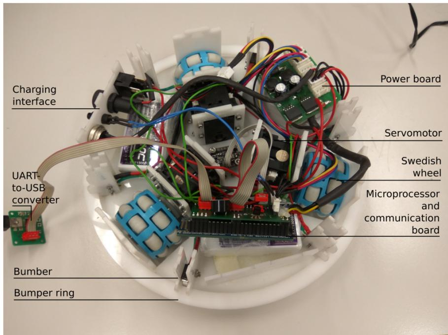
Figure 1: Image of the Omnirobot without top cover
