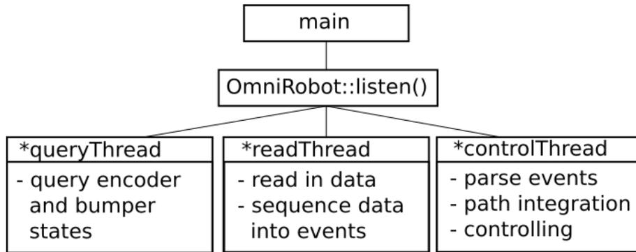
Figure 7: Schematic of the thread setup used for data acquisition and controlling
