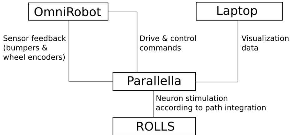
Figure 10: Schematic of the interfaces intended to be used in this project
