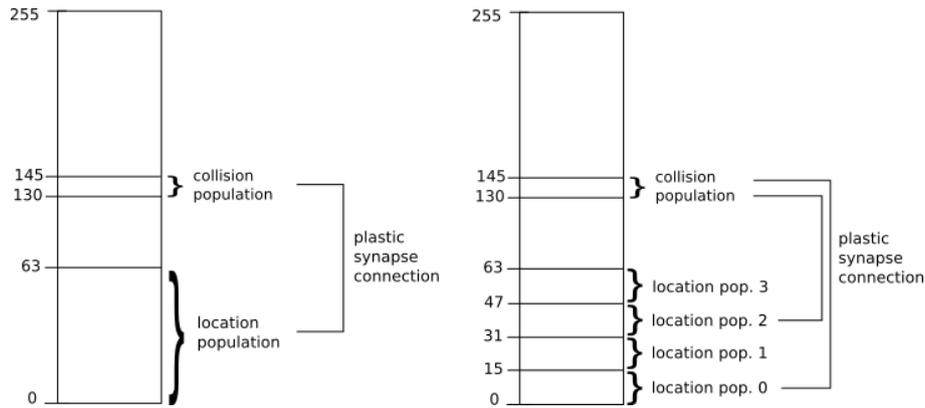
Figure 12: Illustration of the architectures used for the ROLLS experiments. During the first experiment, one location population was used (left). It was later increased to four (right) in a second experiment.
