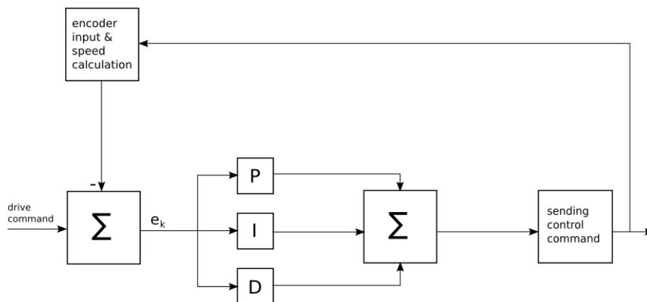
Figure 6: Schematic of the PID controller implemented in this project
