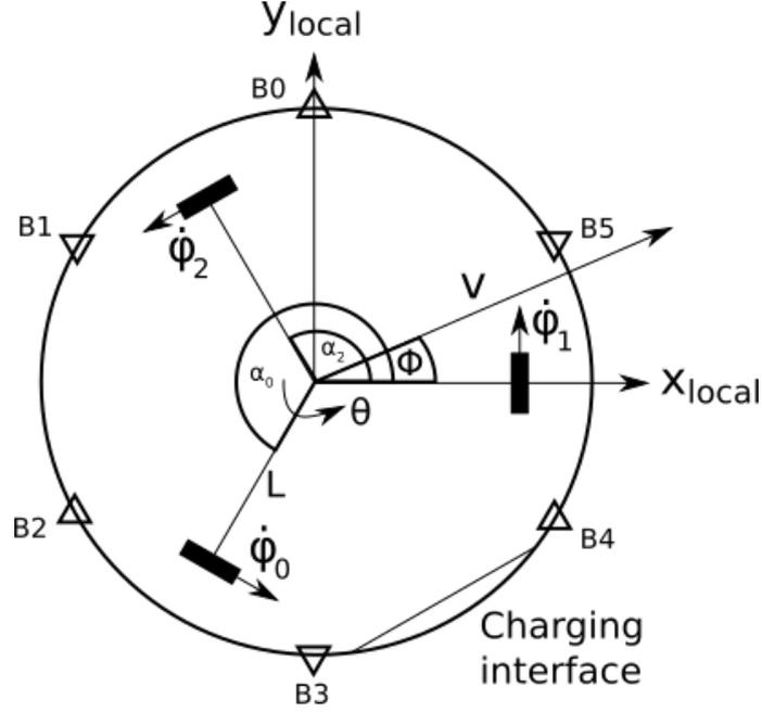
Figure 4: Schematic of the Omnibot with its wheels,  $\dot{\phi}_i$  and bumpers  $B_i$
