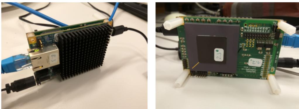
Figure 2: Image of the parallella board during operation (left) and the ROLLS neuromorphic processor mounted on its backside (right)
