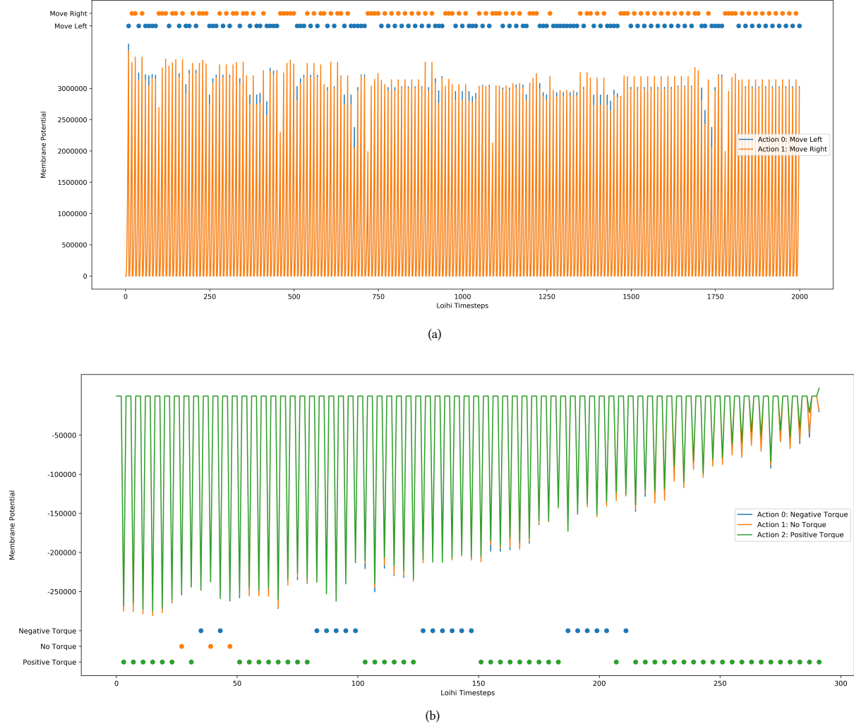
Figure 5: Output neuronal activity for CartPole (a) and Acrobot (b) recorded for one episode on Loihi. Horizontal axis: the number of time steps of the episode multiplied by the simulation time of each trial, listed in Table 2. The dots indicate which action was selected at each time step, based on neuron with the higher membrane potential. In the example runs shown here, the CartPole episode lasted 200 time steps (reward = 200); the Acrobot episode lasted 72 time steps (reward = -72).
