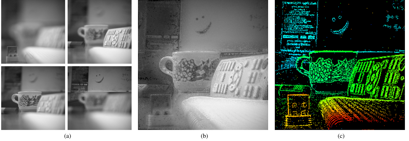
Fig. 4. An example scene imaged by our system ?? shows four images extracted during a focal sweep illustrating the narrow DoF of our system ?? shows an extended depth of field image (all points are in focus) ?? shows a depth map with 64 levels as captured by our system.
