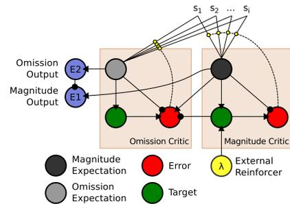
Fig. 5. **The differential outcomes Critic.** TD value expectations for Magnitude and Omission Critics output to relay nodes (expectancy dimensions E1 and E2). The relayed activation of E1 and E2 are used as Actor inputs.
