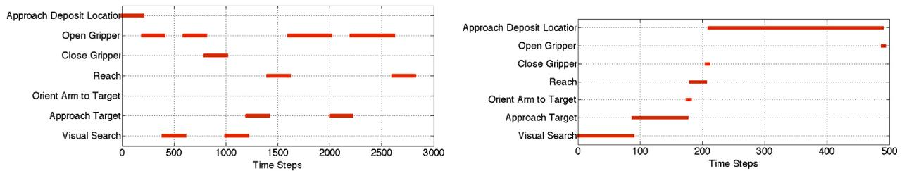
Fig. 5. Timings and Sequences of Elementary Behaviors of the Youbot. Left: During exploration. Right: Performing the Rewarding Sequence.
