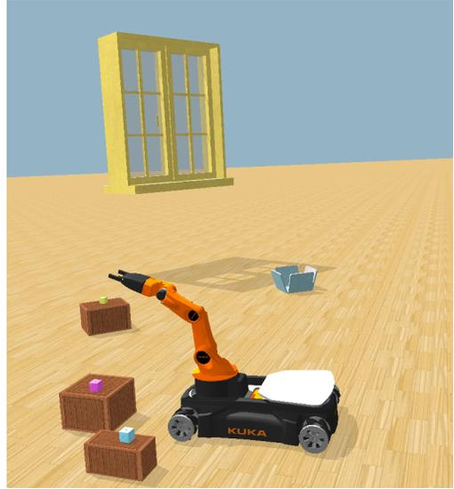
Fig. 1. The simulated YouBot and the environment, in which learning takes place. The task of the robot is to bring colored objects to the grey box.
