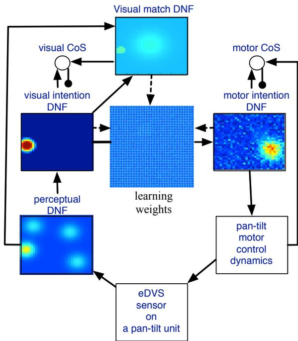
Fig. 1: The DNF sensory-motor map learning architecture. See text for details.
