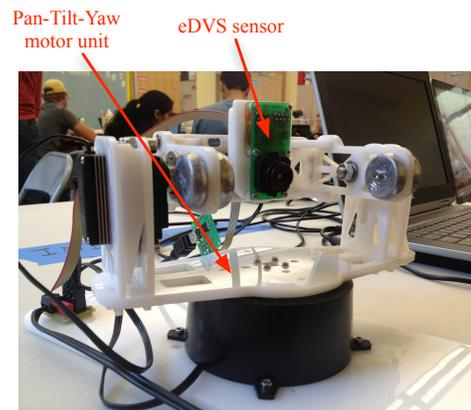
Fig. 3: The DVS sensor mounted on a pan-tilt motor unit.
