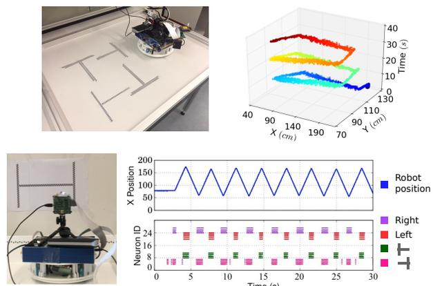
Fig. 6. Real-time real-world experimental results on an omnidirectional robot. We mount the silicon retina and neuromorphic processors on the robot. The output neurons on-chip send out events to drive the robot's motors to go either forward, backward, left, or right. Up: Robot navigates in the arena by recognizing the surface markings on the ground. Down: The robot keeps changing between left and right movements.
