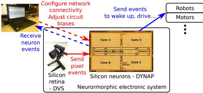
Fig. 1. The neuromorphic electronic system consists of DVS sensors and DYNAP chips. A computer is used to configure the sensors and chips, monitor their activities, or perform learning algorithms. Once a network is set up, or the learning stops, the computer can be disconnected. The perception and processing in neuromorphic sensors and processors are ultra-low-power.
