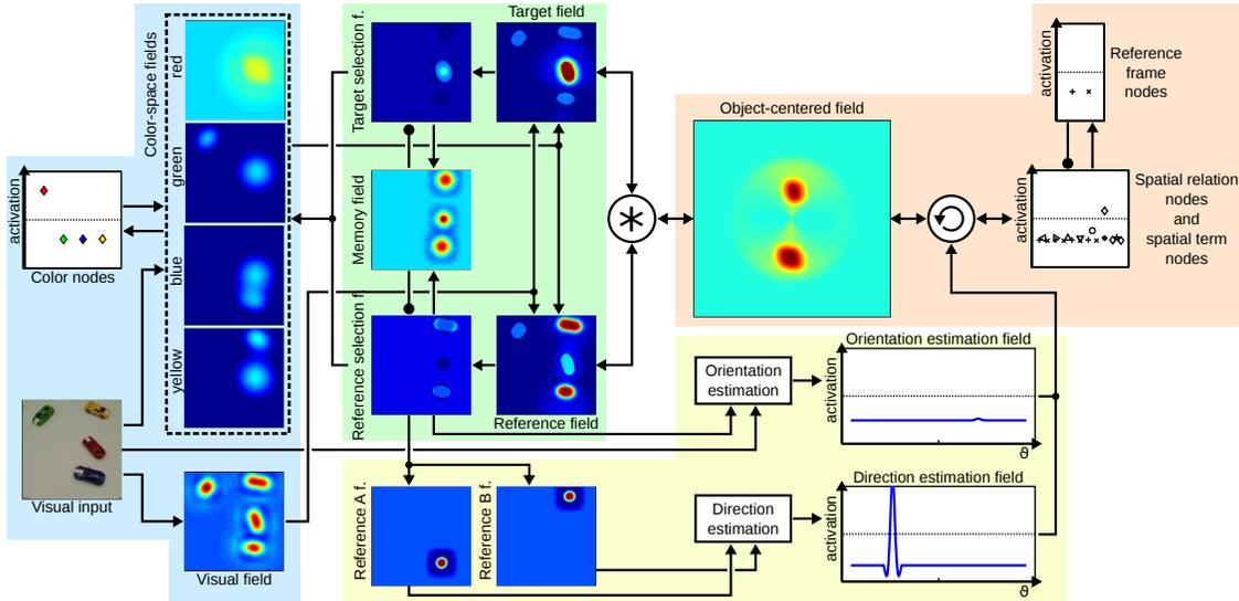
Fig. 1. The neural dynamic architecture is shown together with a snapshot of the activation patterns in the different Dynamic Fields. The snapshot is taken at the final stage of answering the query “what is between the blue and the yellow object?”. The response of the model can be read off the color nodes, the elevated activation level of the node for red designating the red object.
