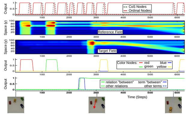
Fig. 4. Time courses of inputs and activation levels for the task “What is between the red and the green car?” The activation of the target field and the reference field is summed along the horizontal spatial dimension.
