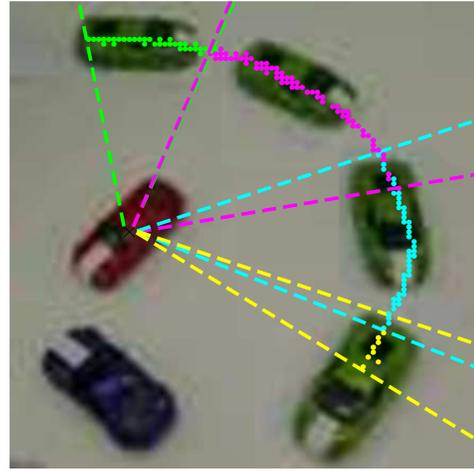
Fig. 7. The target object (green car) was presented at different positions along an imaginary circle. Four samples of visual input are show. Colored dots near the green cars indicate the positions of peaks in the object-centered field for different inputs. In the sector demarcated by green dashed lines, the model responds “viewer-centered behind”. Analogously, the other response sectors are marked: magenta for “intrinsic behind”, cyan for “viewer-centered right”, and yellow for “intrinsic left”.
