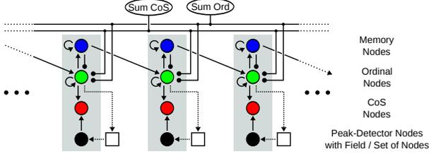
Fig. 2. Schematic of the nodes for sequence generation. Each stage in a sequence is represented by a memory node, an ordinal node, a condition-of-satisfact (CoS) node, and a peak detector node which receives input from a Dynamic Field. Each ordinal node receives inhibitory input from the weighted sum over the output of all CoS nodes and from the ordinal nodes.
